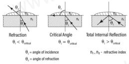
In the **MA881**, light from an LED passes through a prism in contact with the sample. An image sensor determines the critical angle at which the light is no longer refracted through the sample. The **MA881** automatically applies temperature compensation to the measurement and converts the refractive index of the sample to Invert sugar concentration in units of percent (by weight).
