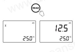
**Note:** The ATC tag blinks and automatic temperature compensation is disabled if the temperature exceeds the 10-40  $^{\circ}C$  / 50-104  $^{\circ}F$  range.
