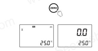
Gently absorb the ZERO water standard with a soft tissue. Use care not to scratch the prism surface. Wipe off the surface completely. The instrument is ready for sample measurement. *Note:* If instrument is turned off the calibration will not be lost.
